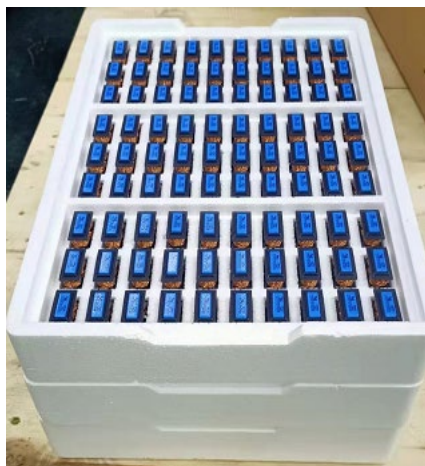
Picture 1: Previous package Polystyrene tray in cardboard box
